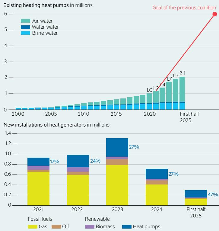
Note: Only heating heat pumps for water-based heating systems. Pure air-to-air heat pumps (air conditioning units) are not included here.
